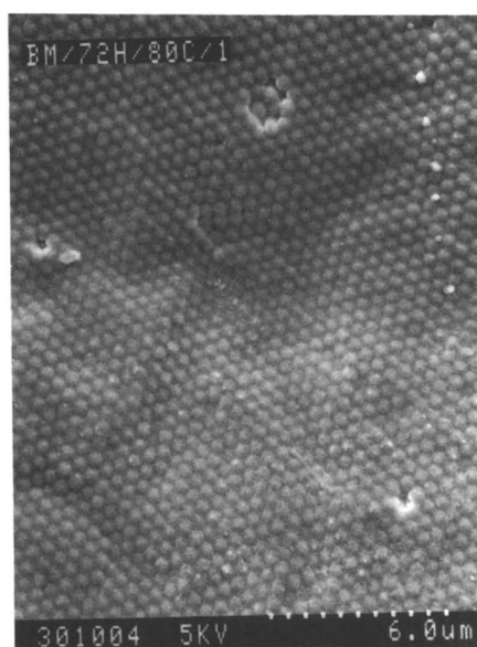
Figure 5 SEM of a PBMA film's polymer-air interface showing particulate close packing.
