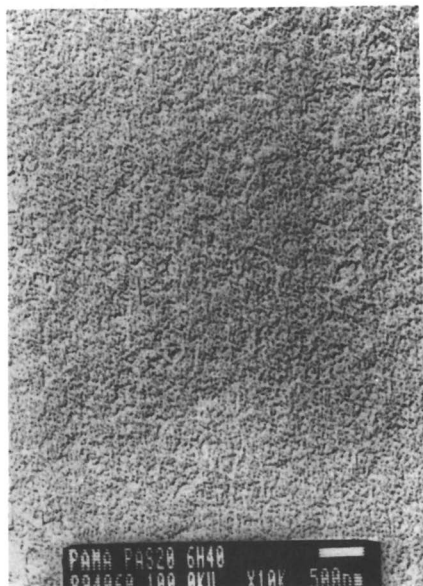
Figure 2 Featureless FFTEM of a PAMA film's cross-section.
